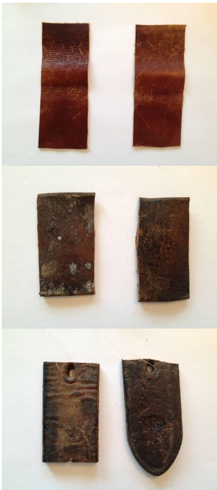
Figure 6. Silicone oil: control samples and post treatment. Samples to the left are control samples. Top: type 1, middle: type 2, bottom: type 3. Photo: Lena Ludwick 2012
