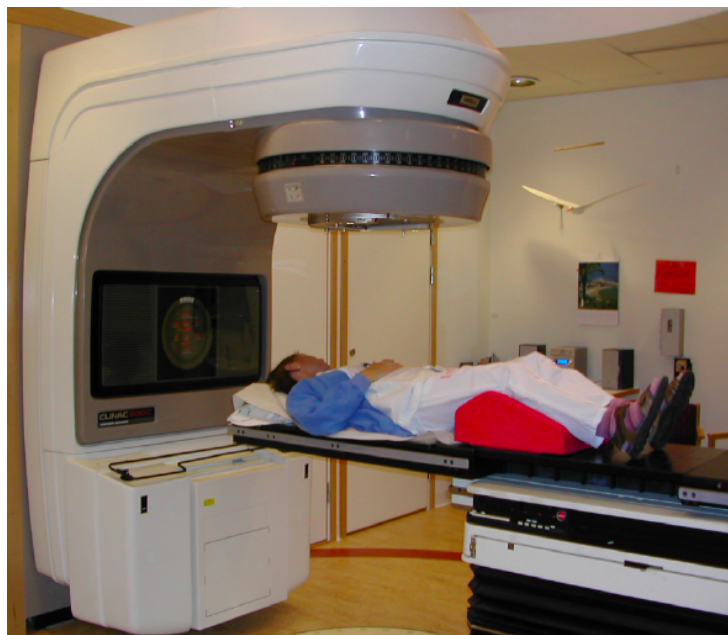
Figure 3. Linear accelerator used in external beam radiation therapy.
