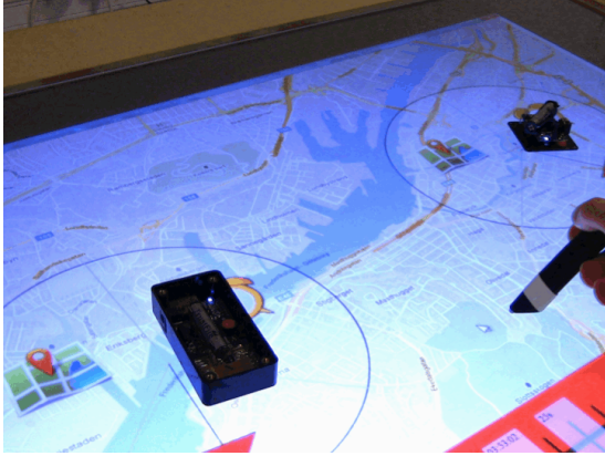
Figure 1: A tangible tabletop map-based application for TUI and pen-based interaction with Google Maps.
