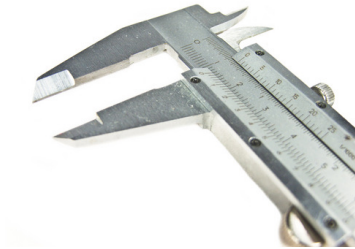
Fig. 5.5 A metric Vernier instrument. How can we transfer this idea into high-resolution digital time measurements?
