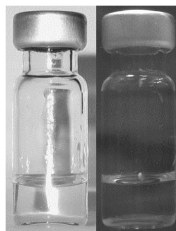
Figure 10. A PEG-containing non-birefringent lipidic sponge phase. Left: No polarization showing a homogenous phase; Right: under polarizers.
