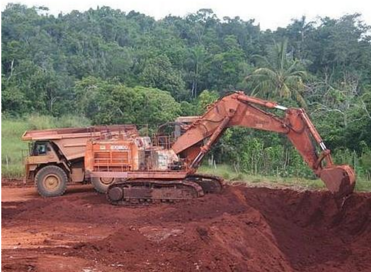
Picture 4.1 Mining operation in Manchester, Jamaica mining bauxite soil for alumina production
