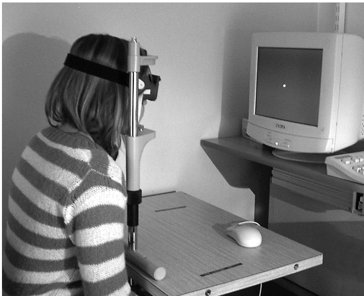
Figure 4b. Child sitting comfortably 53 cm from the computer screen during the recording procedure.
