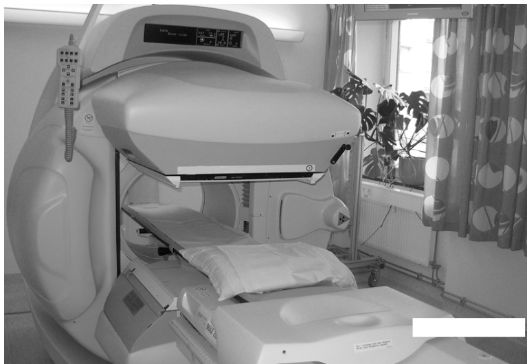
Figure 5. A gamma camera with capability to acquire planar whole-body and tomography images.
