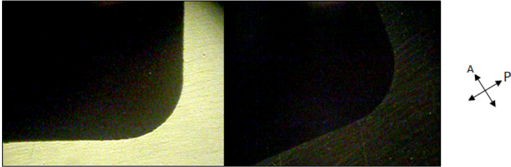
Figure 4.2: Photograph of a cell with cell gap of 1.8 \mu\text{m} containing BC nematic material at 90 \text{ C} . The cell is inserted between crossed polarizers with optic axis at 45 (left) and (right) 0 with respect to the direction, of the polarizer. Dc electric field of 2\text{V}/\mu\text{m} is applied to the cell. As seen, the dark state of the pixel a) is excellent, and b) it does not change when the cell is rotated at 45 .
