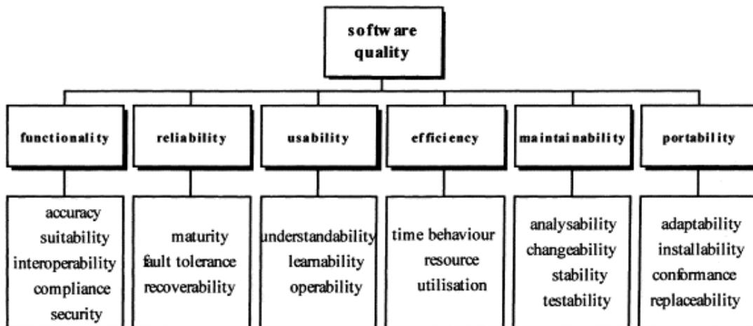
Figure 9 - Software quality characteristics [24]
