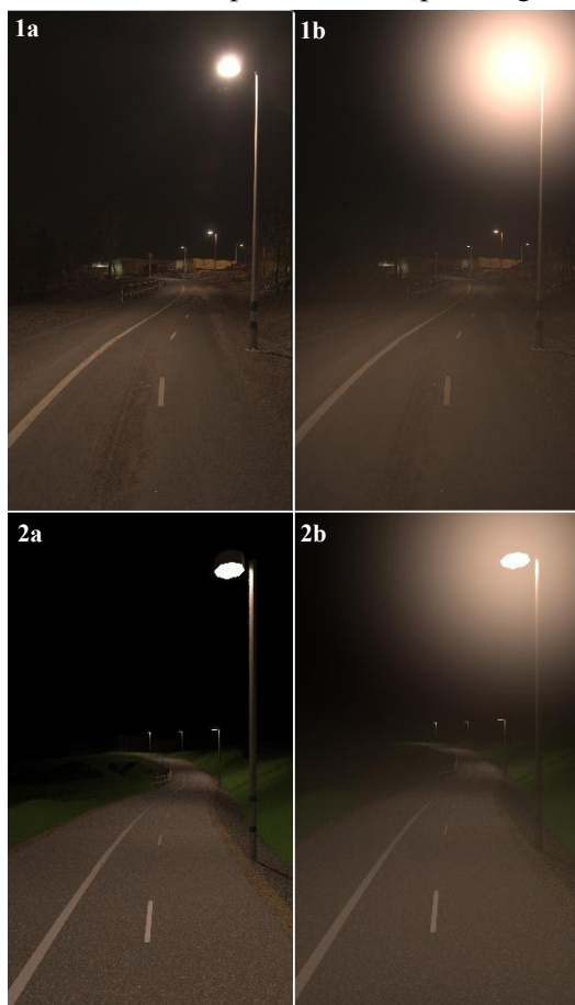
Figure 1.4: The second column in the image arrangement shows the filtered images. The upper row depicts a photo and the lower row shows the render.
