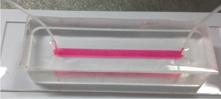
Figure 3.1: Photograph of a microchannel of the type used in our experiment. The channel is molded in a block of PDMS plastic. In the picture the channel is filled with dye. To the left and right are inlet/outlet tubes. The channel is ca 5 cm long.
