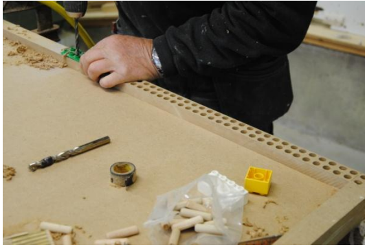
The process of building a prototype in MDF, scale 1:1.
