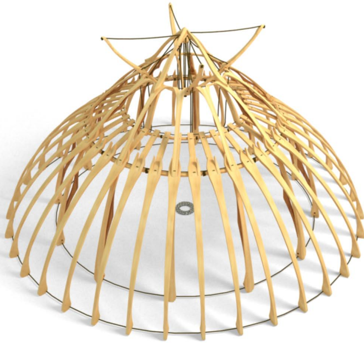
Figure Nr.: 50 - Visualization, design of the Sprout 'c', the completed, opened shape.
