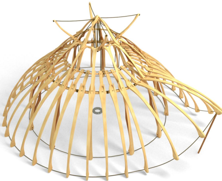
Figure Nr.: 51 - Visualization, design of the Sprout 'c', the completed, opened shape with raised entrance.
