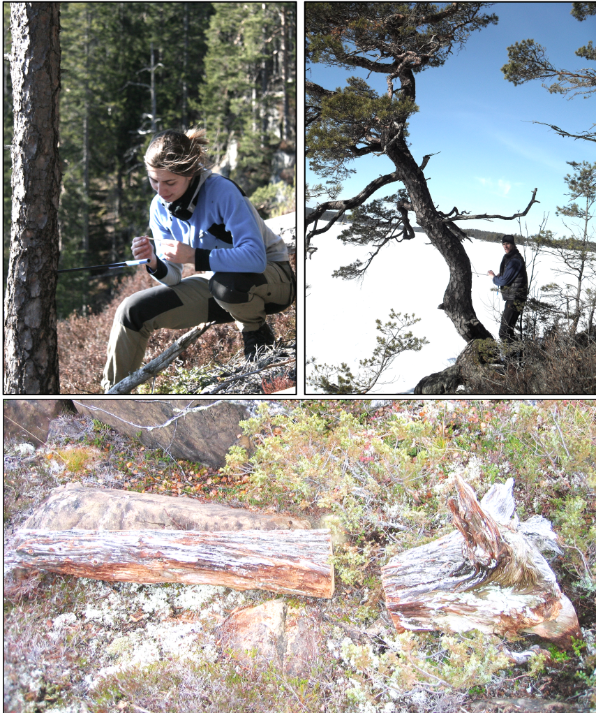
Figure 8. Data sampling with increment corers top panels, and sawn discs from deadwood on the ground, bottom panel.
