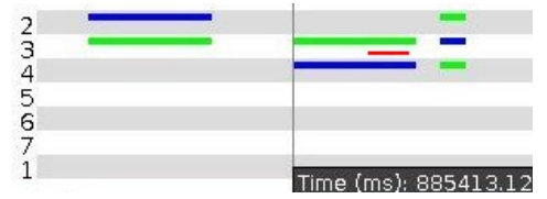
(b) Incorrect acknowledgement: Node 3 checks the EDC for one sender node that gives routing progress but acknowledges the packet from the other sender node that does not give routing progress.
