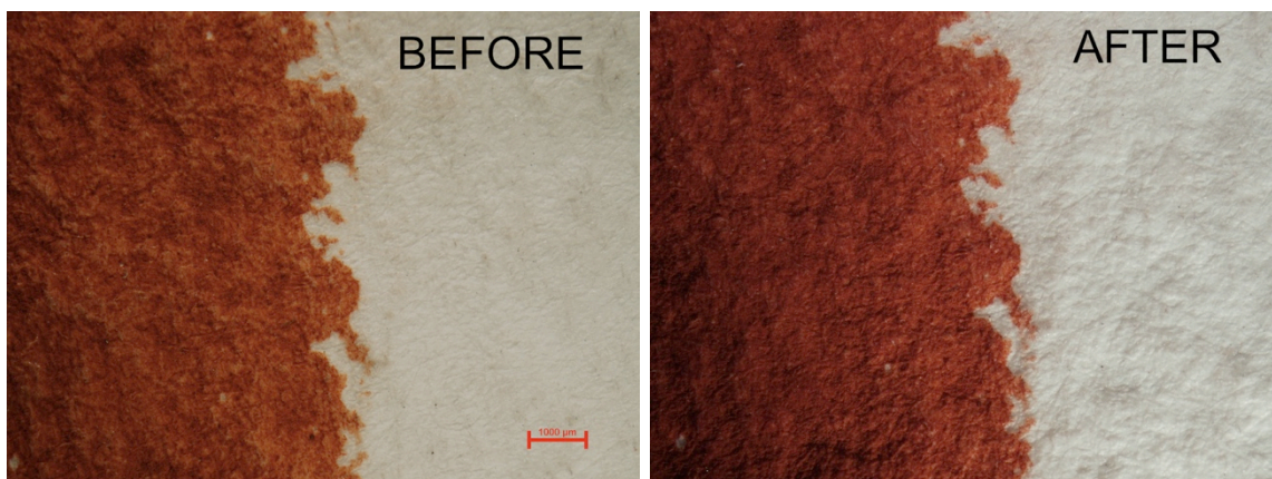
Fig.16: Example of category 1: No noticeable lateral migration. M4:Hi I before and after immersion wash
