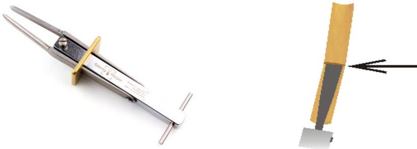
At the moment I use number 118 shape. The shaping machine (there are many brands of them) is superior in quality to hand shape tips because the gouged cane sits flat, not folded, and the angle of the blade is set ensuring perfectly even sides. This is crucial in helping reeds vibrate properly once bound onto the staple.
