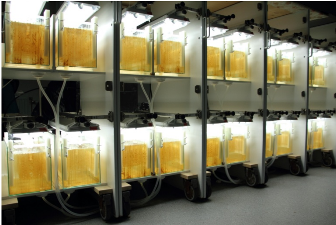
Figure 7 – Aquaria microcosms used for paper III and IV. The glass discs are mounted on the long-sides of the aquaria. Photo: Mikael Johansson
