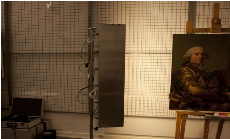
fig.9 Lighting stack(6 X 75 W) with adjustable amount of light, placed on the left side of the painting.
