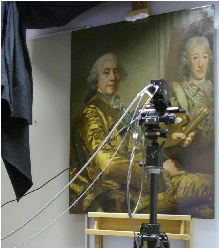
fig.12. Interiordetail: Ramanprobeinvestigation of the Selfportrait 1790, the laboratory at the Institute of Conservation Gothenburg
