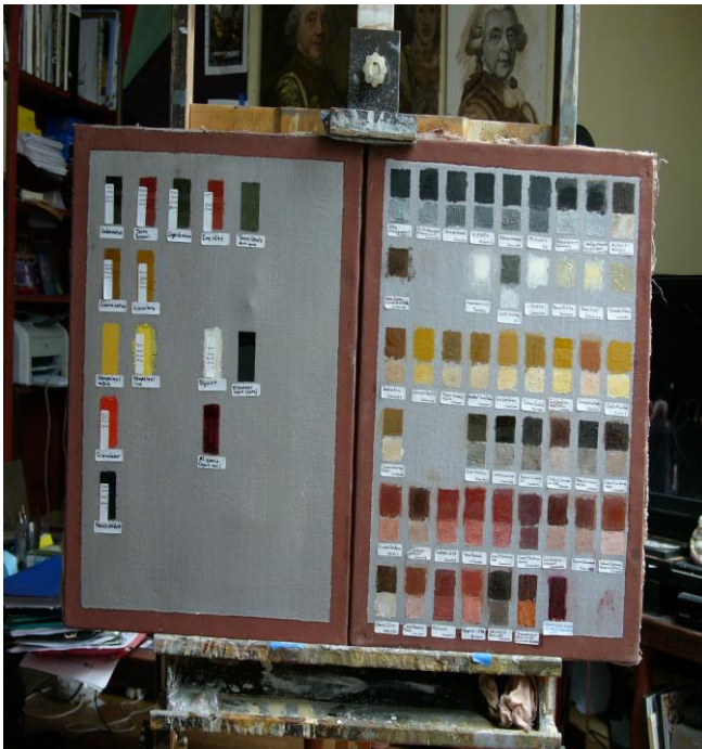
fig 13. Reference tests were performed on color samples on canvas prepared with a traditional doubleground with the Raman probe, Parts of the color samples were covered with a rather thin layer of varnish( in this casea syntetic varnish of ketonetype)
