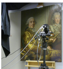
fig.12. Interior detail: Raman probe investigation of the Self Portrait 1790, at the laboratory at the Institute of Conservation Gothenburg
