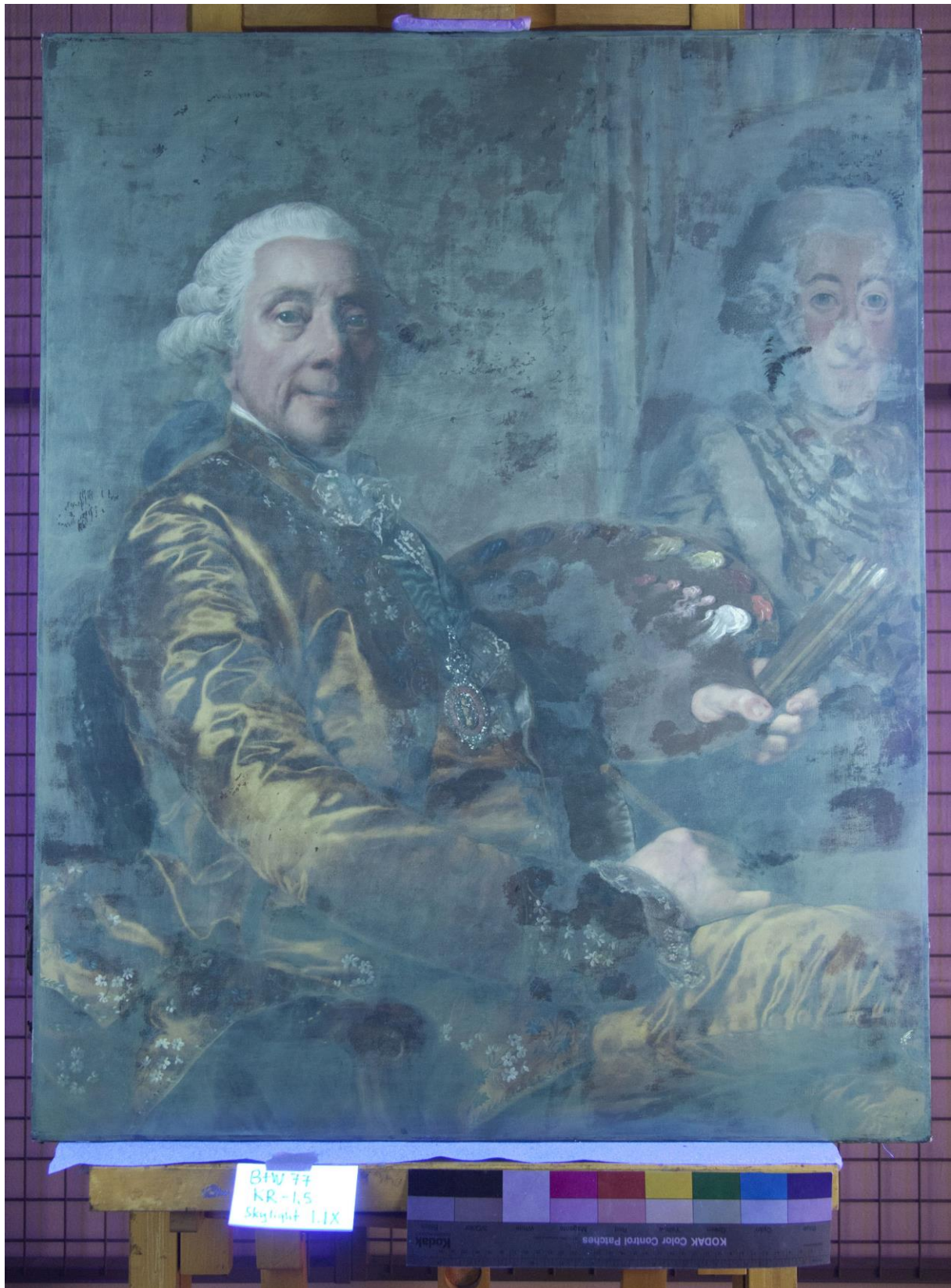
fig.95 UV- induced fluorescence, B+W 77 KR 1,5 Filter, (Skylight 1.1X ).
