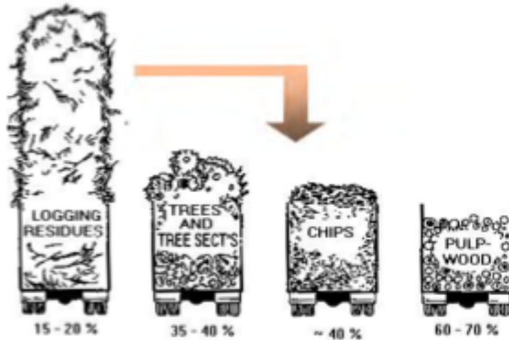
Figure 6: The differences between different types of biomass (Björheden et al., 2010). All loads contain the same amount of biomass, but in different forms they occupy different amounts of space.
