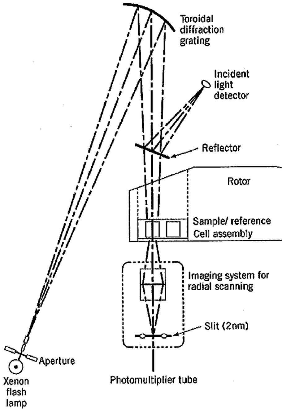
Fig. 11. Optima XL-I Analytical Ultracentrifuge
