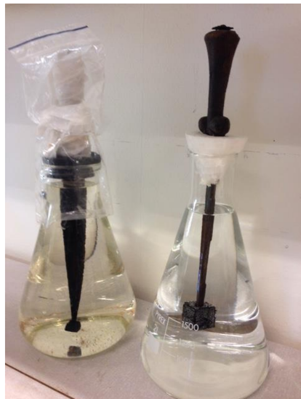
Figure 2: Iron dagger with wooden hilt during desalination with NaOH at SVK.
