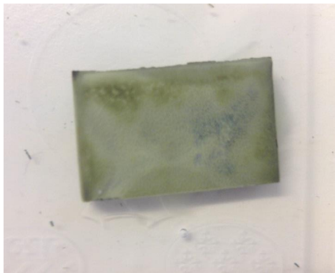
Figure 16: Modern iron in disodium phosphate solutions after 6 weeks.
