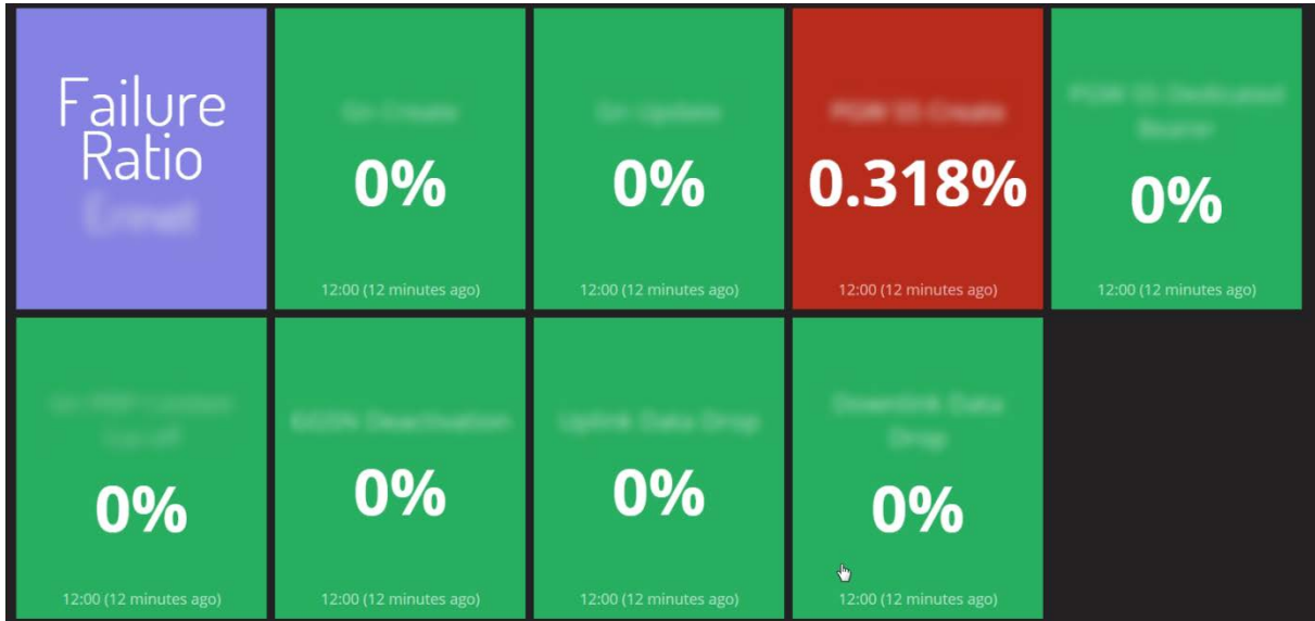
Figure 11: A dashboard containing widgets showing the failure ratio, one of them is pulsating red since the value is over a set threshold
