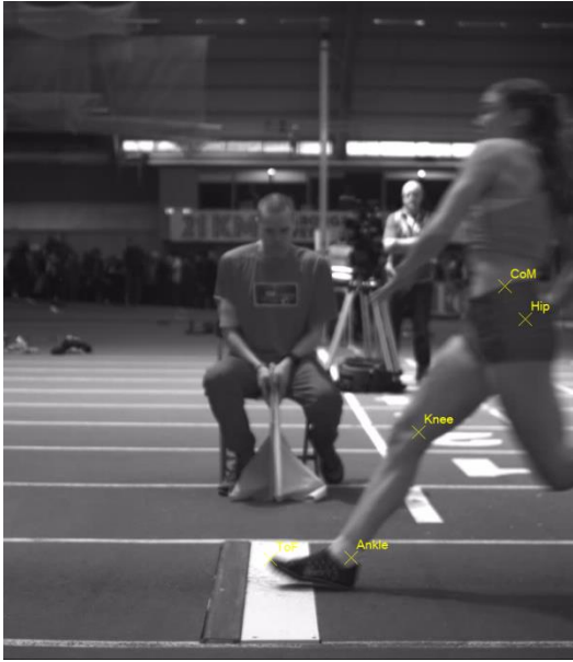
Figure 2. Touchdown frame with markers for tip of foot, ankle, knee, hip and centre of mass
