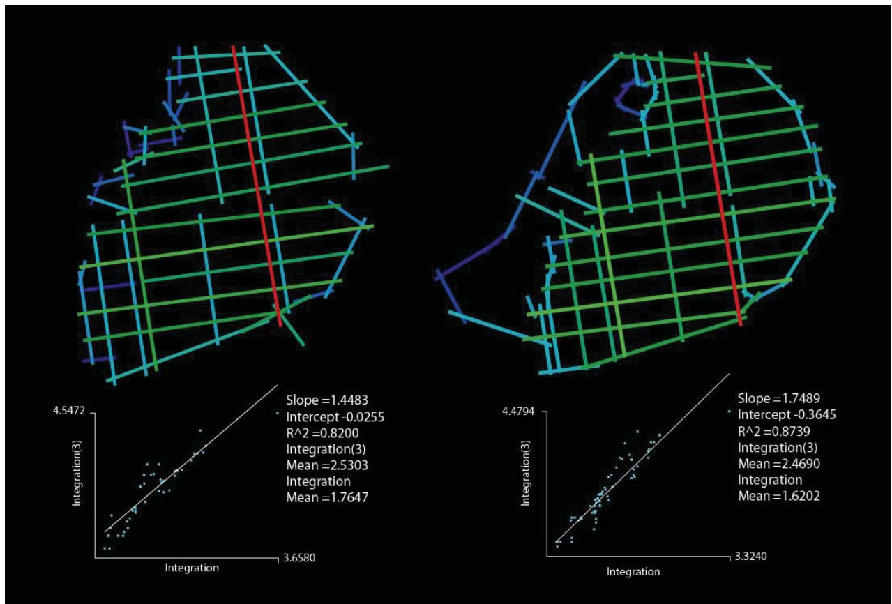
Fig 1: Analyzed axial model and local global scattergram of Gothenburg in 1644 (left) and 1753 (right).
