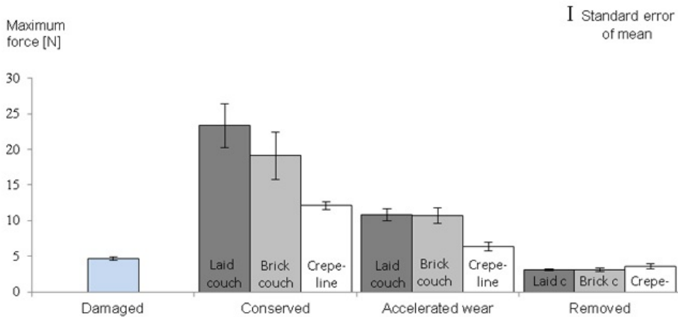
Figure 15. The maximum force at break of surrogates with tear without any conservation and after conservation with three different methods, after being subjected to accelerated wear and after removal of the conservation.
