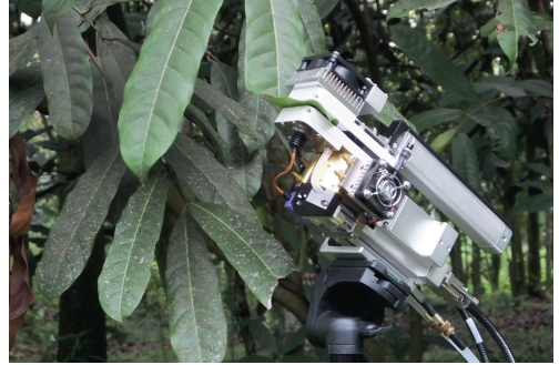
Figure 10. Leaf gas exchange measurement on Carapa grandiflora for Paper IV. Photo by Thomas B. Hasper.
