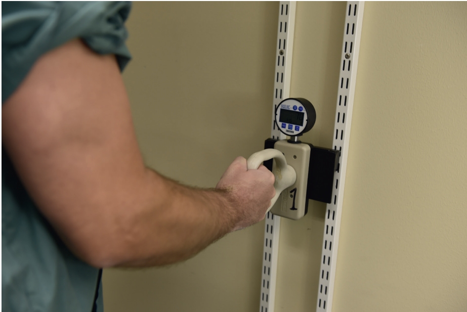
Figure 24. Measurement of peak torque strength of the right wrist in supination, standing with the elbow fixed to the body and in 90° flexion. Measurement technique developed by Peter Axelsson. Photo: Tommy Holl.
