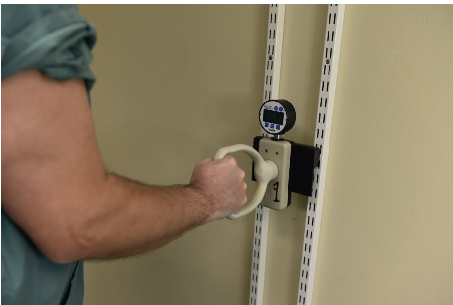
Figure 51. Measurement of peak torque strength of the right wrist in pronation, standing with the elbow fixed to the body and in 90° flexion. Measurement technique developed by Peter Axelsson. Photo: Tommy Holl.
