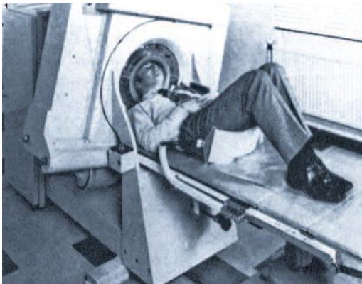
Figure 6. The first clinical prototype EMI brain scanner installed at Atkinson Morley's Hospital, in London, England 1971.
