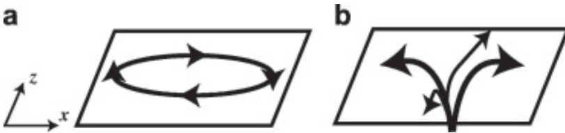
Figure 13. Decomposition of the interfacial velocity vector into (a) solenoidal and (b) irrotational components. (Figure 4 in Hasegawa and Kasagi [2008])
