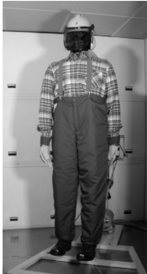
Figure 1. Prototype of a physiologically optimised protective clothing system for users of hand held chain saws during the tests with the thermal manikin "Charlie".
