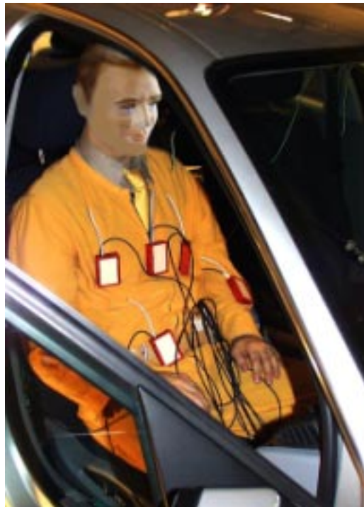
Figure 5. Dummy Representing Suit for Simulation of huMAN heatloss (DRESSMAN). Here six of the velcro fastened RST-meters can be seen. The white wires keep the air temperature sensors.
