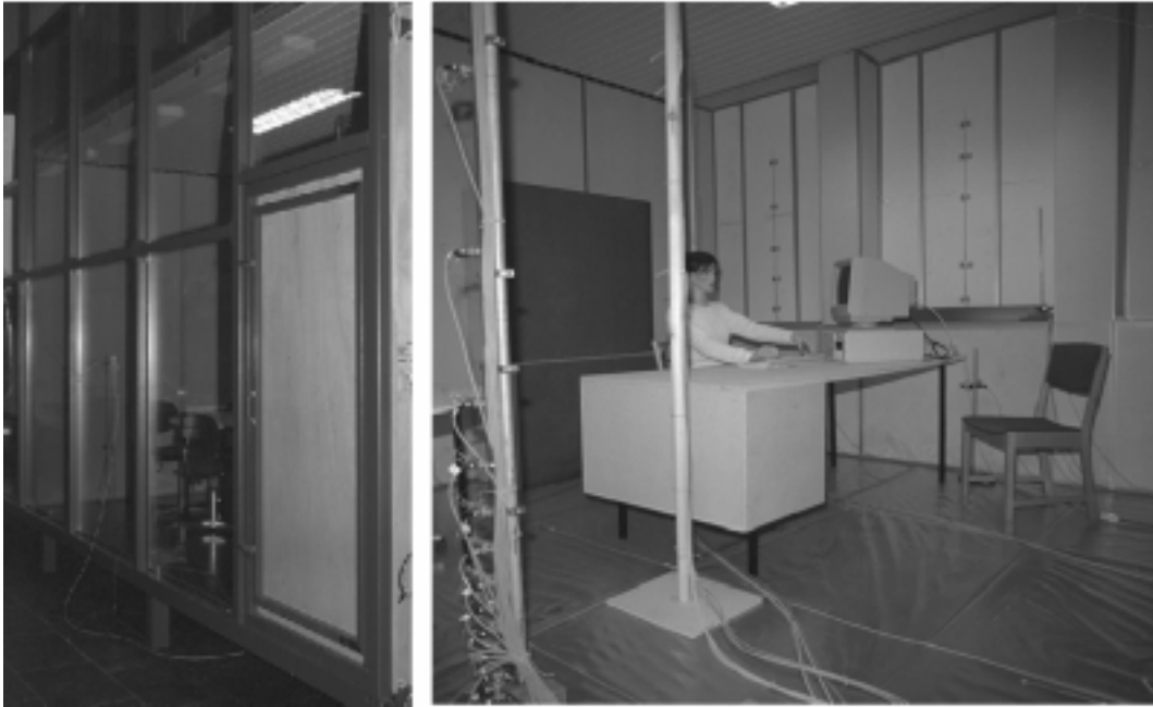
Figure 3. CASE 2. Personal exposure to emission from a carpet in a typical cell office. Left: Mock-up seen from outside. Right: Mock-up seen from inside.
