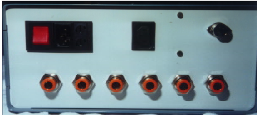
Figure 3. The rear side of the artificial lung, showing the six connectors. Two to inhaling and exhaling to and from the manikin. Two to and from the pump, one for inhalation of fresh air, and finally one to the analysing equipment. On top right is seen the connector to the computer from where the breathing volume and frequency are controlled.
