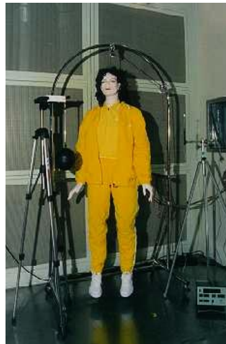
Figure 2. An experiment stand intended for testing clothing insulation of a nude manikin resting in standing posture. Determination of I_a
