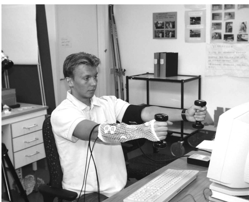
Figure 4. The posture used to assess the reference voluntary electrical activity (RVE) for the trapezius muscles in Studies I & III.
