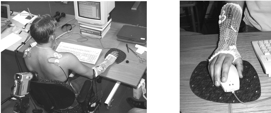
Figure 3a and 3b. Showing the position of the EMG electrodes, the electrogoniometer and the force-sensing mouse in the laboratory studies (Studies I & III).
