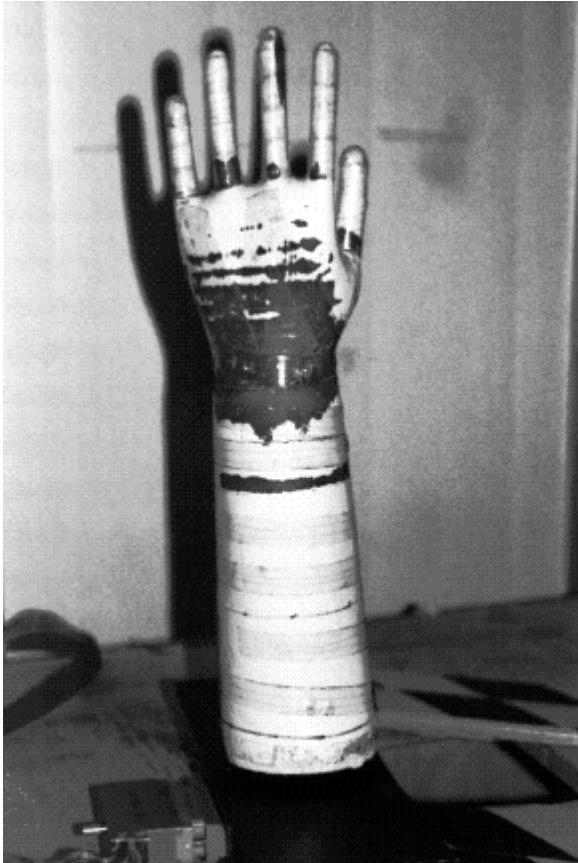
Figure 14. An electrical hand model for measurement of thermal insulation.
