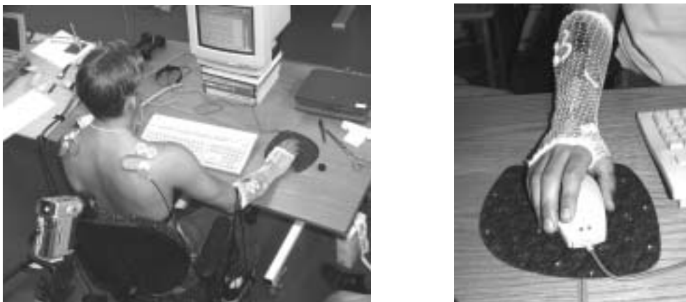
Figure 9. The position of the EMG electrodes (left), the electrogoniometer and the force-sensing mouse (right) in Studies I and III.
