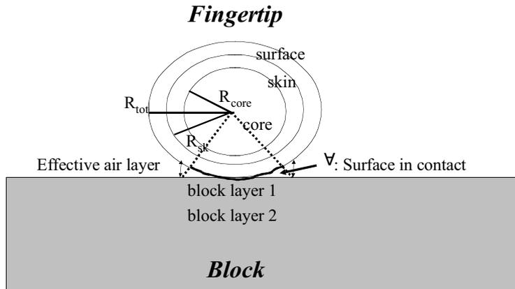
**Figure 2.** Schematic presentation of the model to simulate contact cooling of the fingertip. All parameters are denoted in the text. The finger is represented as a cylindrically shaped object. The grey square represents part of the block (CS84).
