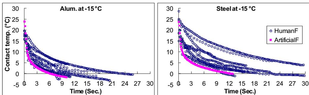
**Figure 22.** Comparisons of cooling curves between the artificial finger and human finger where touching cold metallic surfaces at  $-15$  °C.
