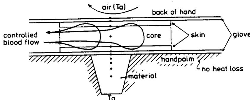
**Figure 3.** Schematic representation of the cooling model according to Lotens. It contains 11 compartments or nodes (5 nodes for the material, 2 for the gloves, 3 for the hand and 1 for environmental air).
