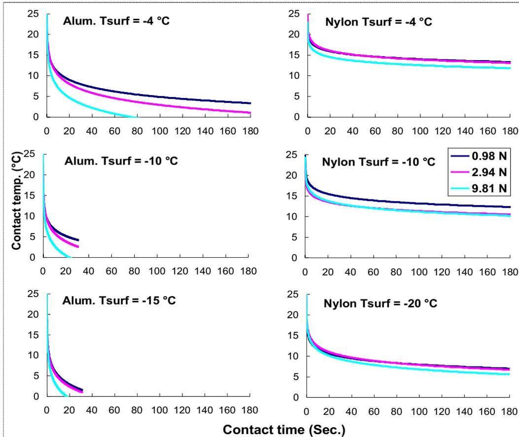
**Figure 9.** Contact temperature versus cold touching duration of aluminium and nylon with 3 pressure (0.98, 2.94 and 9.81 N) at different surface temperature.
