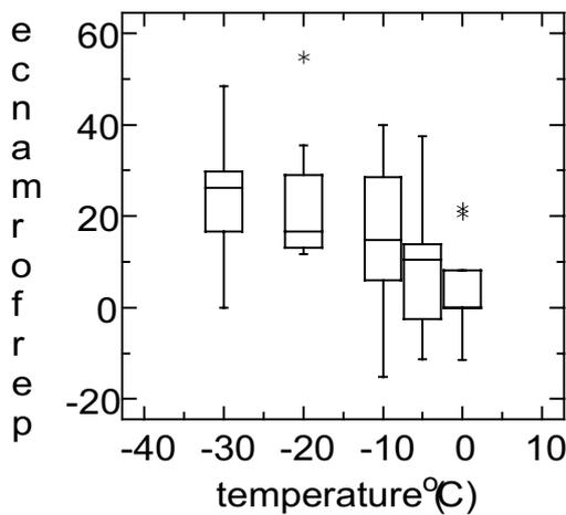
**Figure 14.** Relationship between performance reduction and air temperature.
