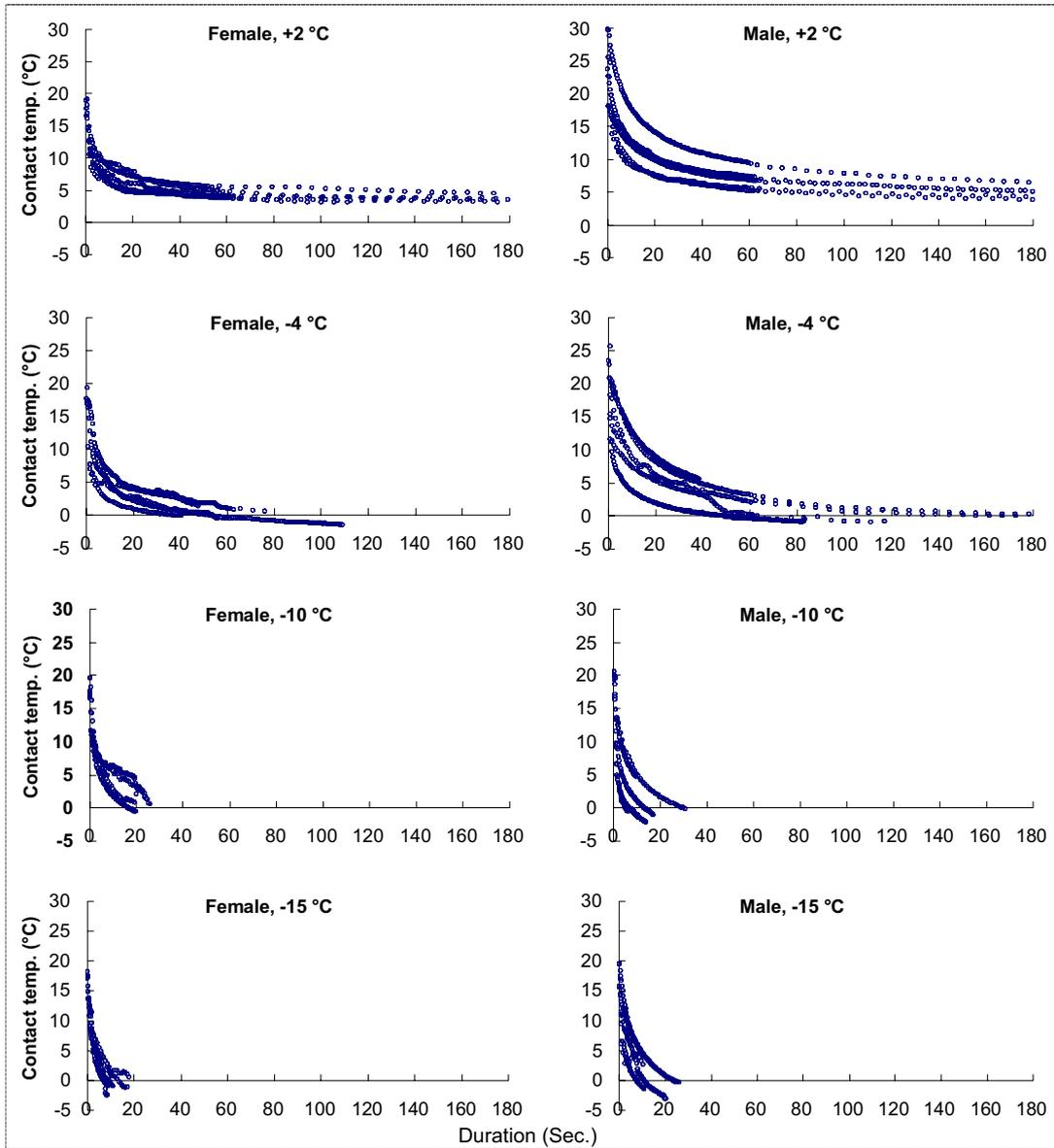
**Figure 8.** Contact temperature versus cold touching duration of aluminium with a pressure of 9.81 N at 4 different surface temperature
