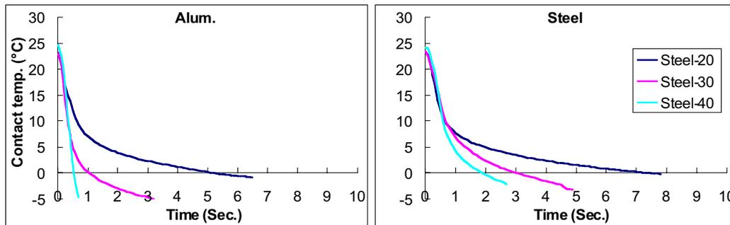
**Figure 21.** Change in  $T_C$  of artificial finger in contact with metallic surfaces (alum. and steel) at temperature  $-20$ ,  $-30$  and  $-40$  °C.
