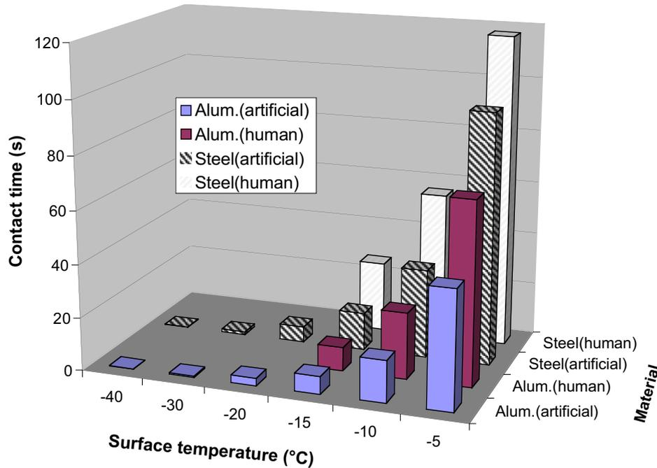
**Figure 23.** Contact time for  $T_C$  to reach freezing criterion ( $0\text{ }^{\circ}\text{C}$ ) at various surface temperatures using the artificial finger under extremely cold conditions:  $T_S \leq 20\text{ }^{\circ}\text{C}$  and both human finger and artificial fingers at  $T_S \geq -15\text{ }^{\circ}\text{C}$ .
