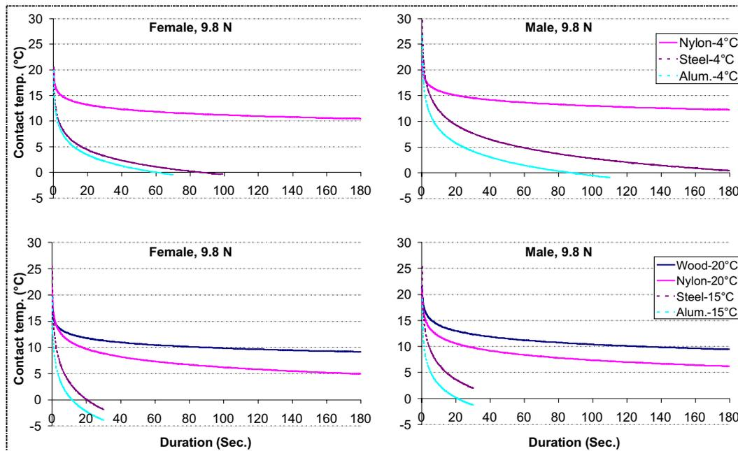
**Figure 7.** Contact temperature versus cold touching duration of 4 materials with a pressure of 9.81 N at  $-4$  and  $-20/-15$ .
