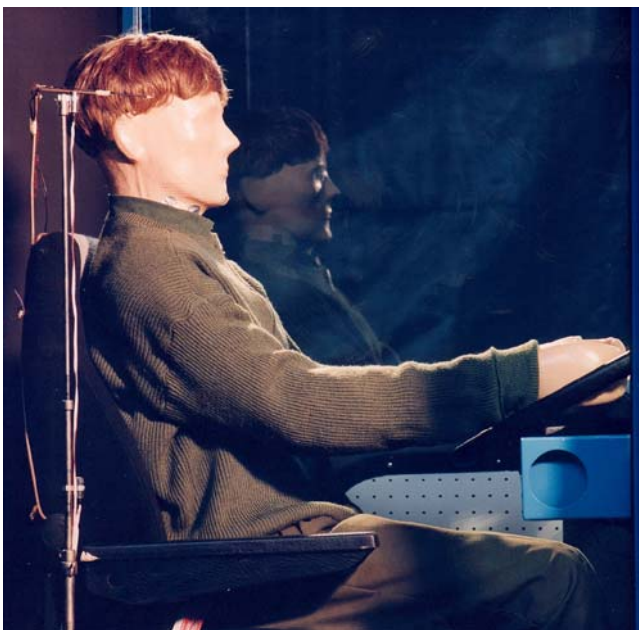
Figure A9. MANIKIN2 in winter clothing inside the cabin simulator with the sensor tree at the right side in the same way as MANIKIN3 in case 3.
