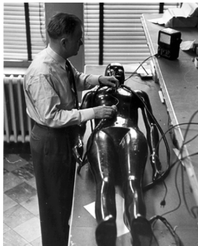
Figure 14. Copper manikin used in studies on body temperature. Photo: H. Corsini. June 1951. Oakland: School of Public Health, University of Pittsburgh. From the Collections of the Pennsylvania Department, The Carnegie Library of Pittsburgh.
