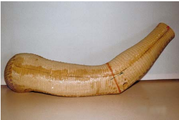
Figure A4. The ready made right arm of MANIKIN2 with the heating wires fixated with glue and the pins taken away, ready for plastic covering.
