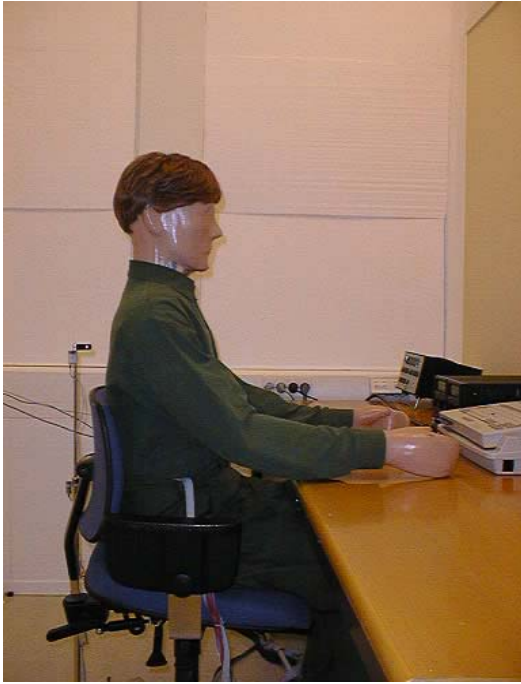
Figure 71. Picture showing manikin and computer in the office room.
