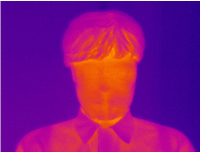
Figure A5. IR image (ThermaCAM PM 515, FLIR Systems AB, www.flir.se ) of the heated face of MANIKIN2, showing the temperature distribution the hair, face and clothes when heated to 34°C.
