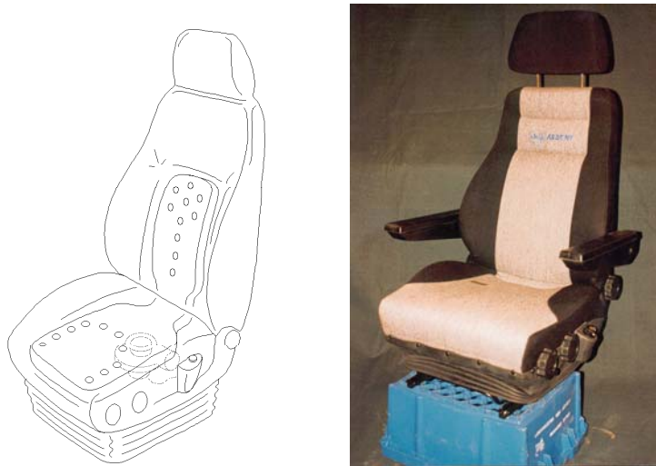
Figure 51. The ventilated seat showed see through view as well as a photo. The fan was positioned in the seat sucking air through channels in the seat and lower backrest.
