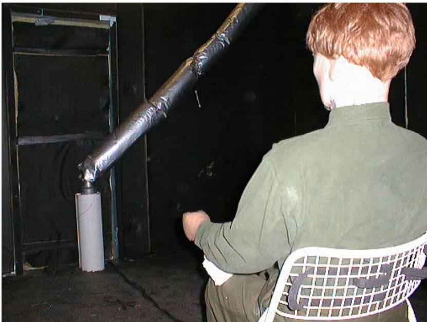
Figure 65. The thermal manikin MANIKIN2 inside the climatic room.
