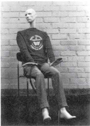
Figure 36. The manikin "Clousseau" used to determine convective heat transfer coefficients.
