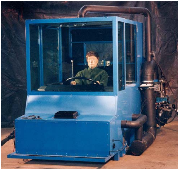
Figure 78. MANIKIN2 inside the cabin simulator exposed to the artificial sun. The two black outlets are visible on the lower back wall.
