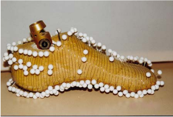
Figure A3. The left foot of MANIKIN2 showing the fixation of the heating wire with pins.
