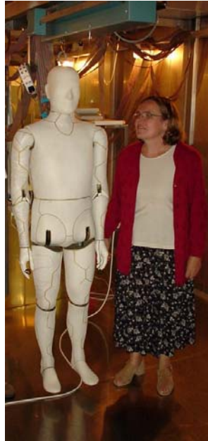
Figure 15. The Finnish sweating Manikin Copelius made during a Nordforsk project developing the TORE series in the 80-ties. (To the right Dr Harriet Meinander, VTT, Finland).
