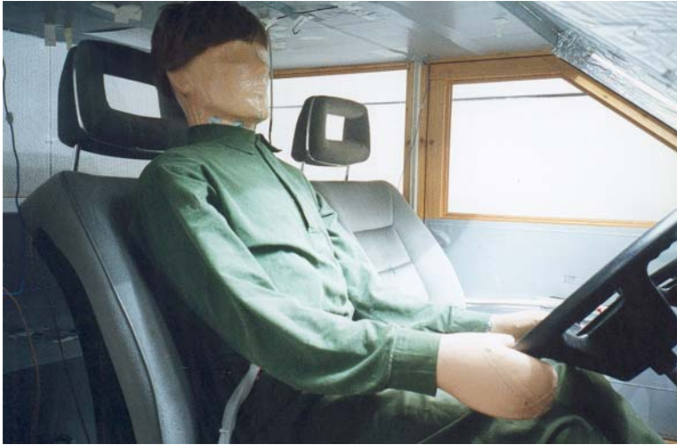
Figure 33. MANIKIN2 inside the test cabin for the warm condition tests.
