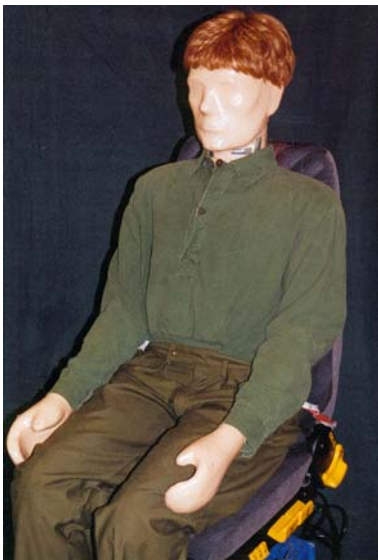
Figure 53. MANIKIN2 positioned in the ventilated seat.
