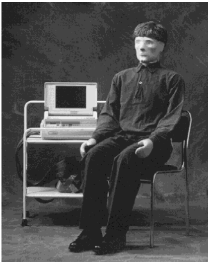
Figure 12. The heated manikin MANIKIN2 with 33 individually controlled zones. This manikin was especially constructed for climate evaluation in 1991.
