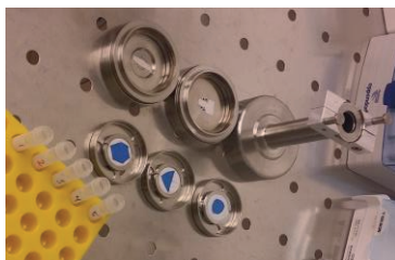
Figure 14. Photo of the three nozzle plates and the three impaction plates of the Dekati 3-stage impactor. The white PTFE-membrane and the blue plastic support can be seen on the impaction plates where the samples have been cut out.
