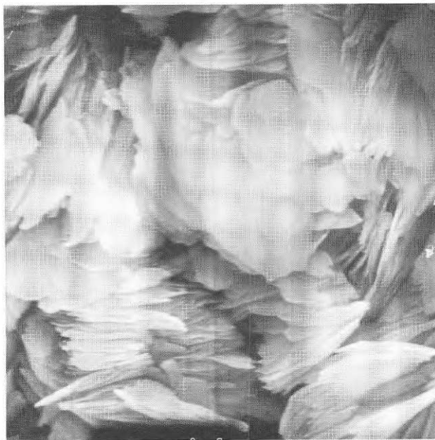
Bro, Södertälje, saltskadad betong, saltformation
