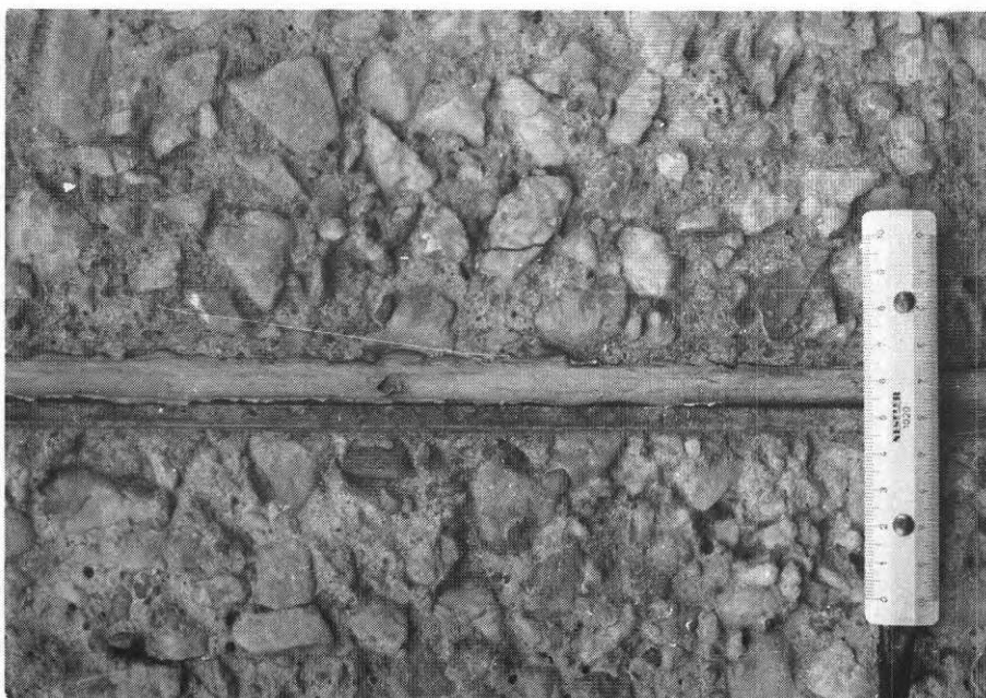
Fig. 96. Planoconcave joint cross section of polysulphide-based jointing compound subjected to a reduction in width of 25 %. Depth-width ratio approximately 1/2.3. There is adhesion between the retainer strip and the jointing compound at the centre of the joint. The strain in the extended diagonal of the lower external edge panel is about 60 %. The strain in depth at the centre of the cross section is about 50 %. The end faces of the joint have been retained by plates of glass which were coated with oil.
