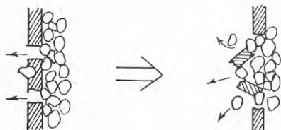
Fig 5.8 Filterrörsbrott p g a korrosion
