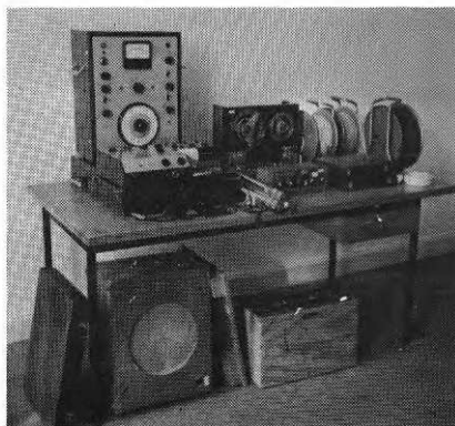
FIG. 2. Equipment for field measurement of sound insulation using the conventional method.
