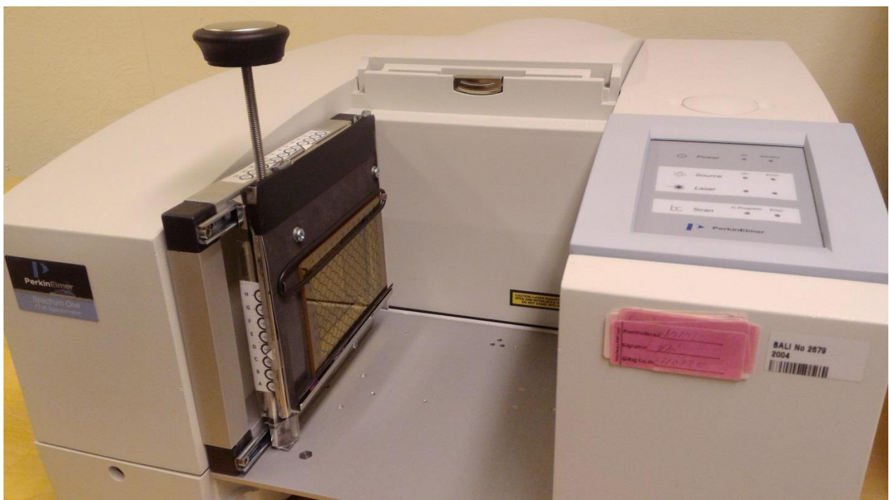
Figure A1. FTIR spectrometer with custom built xy-stage holding a ZnSe well plate as it was used to acquire FTIR spectra of bacterial samples.
