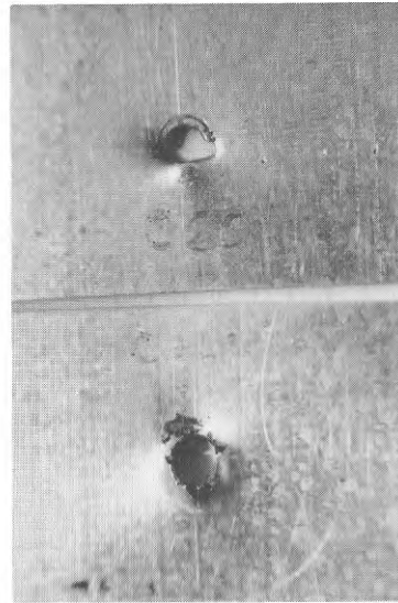
Bild 11. Provkropp C20, C14 P_{\max} = 2200 \text{ N} Def. = 5,0 mm Brottyp SN/SP N = 174.870 spänningscykler
