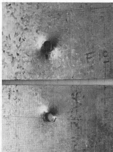
Bild 13. Provkropp F19, F12 P_{max} = 2800 N Def. = 6,0 mm Brottyp SN/S N = 173.940 spänningscykler
