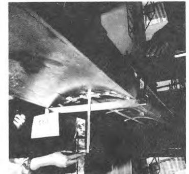
Photograph 1. Upward deflection of bottom flange when element is loaded.
