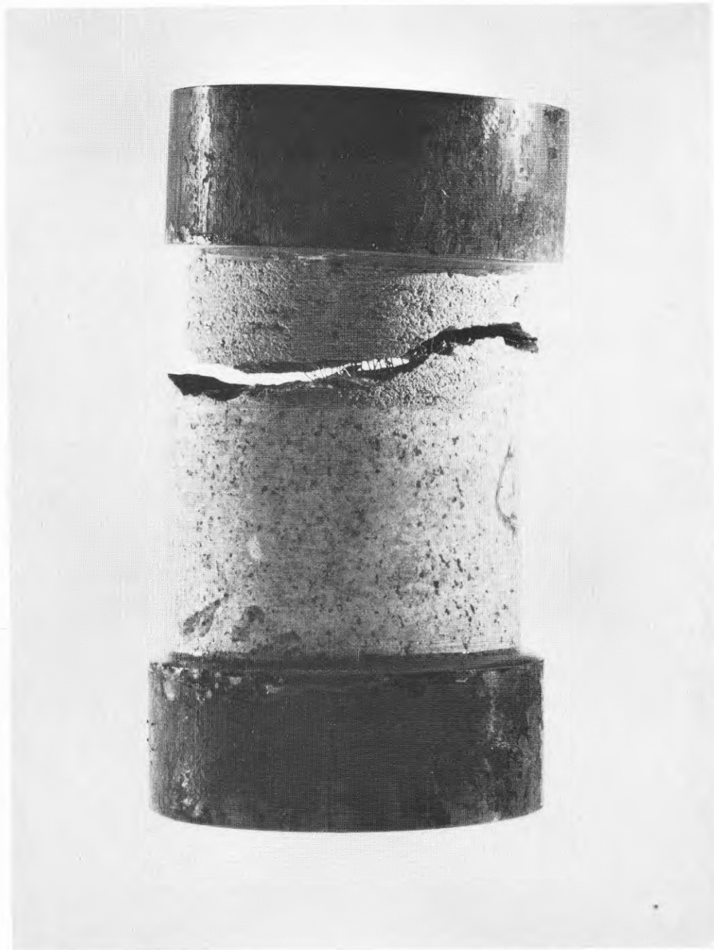
FIG. 40. Vidhäftningsprovning. Kombinerat vidhäftningsbetongbrott. Test of bond strength. Failure in the contact surface and in the concrete.
