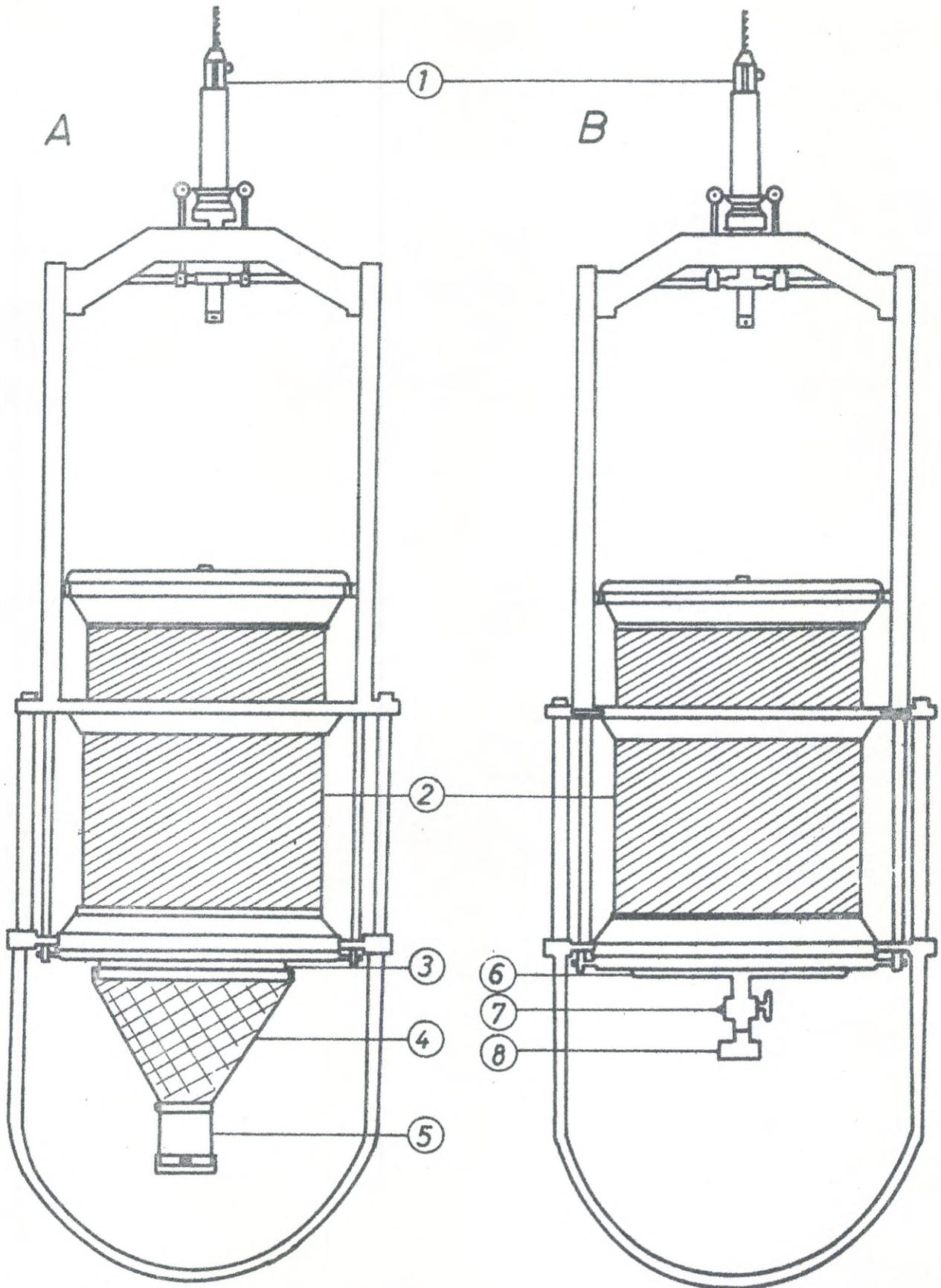
Fig. 1. A plankton sampler with a capacity of 23 litres. A) The sampler is modified for taking zooplankton samples. B) The sampler is modified for taking phytoplankton and water samples (Ackefors, 1971a).
