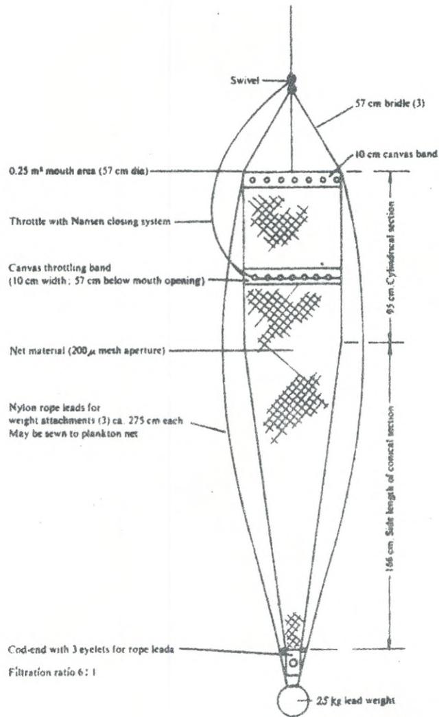
Fig.2. The type of net proposed by Working Party no.2 inside UNESCO for taking smaller mesoplankton (Tranter, 1968).
