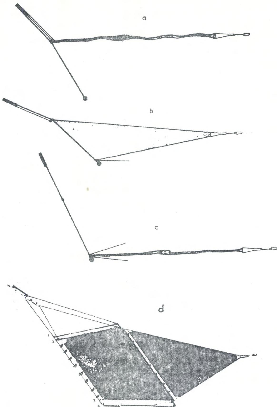
Fig.15. The operation of the rectangular opening-closing trawl; a) the net is payed out to the fishing depth b) the open position c) after closure while it is hauled to the surface d) the rectangular opening-closing trawl in the open, fishing position ( Clarke .1969).
