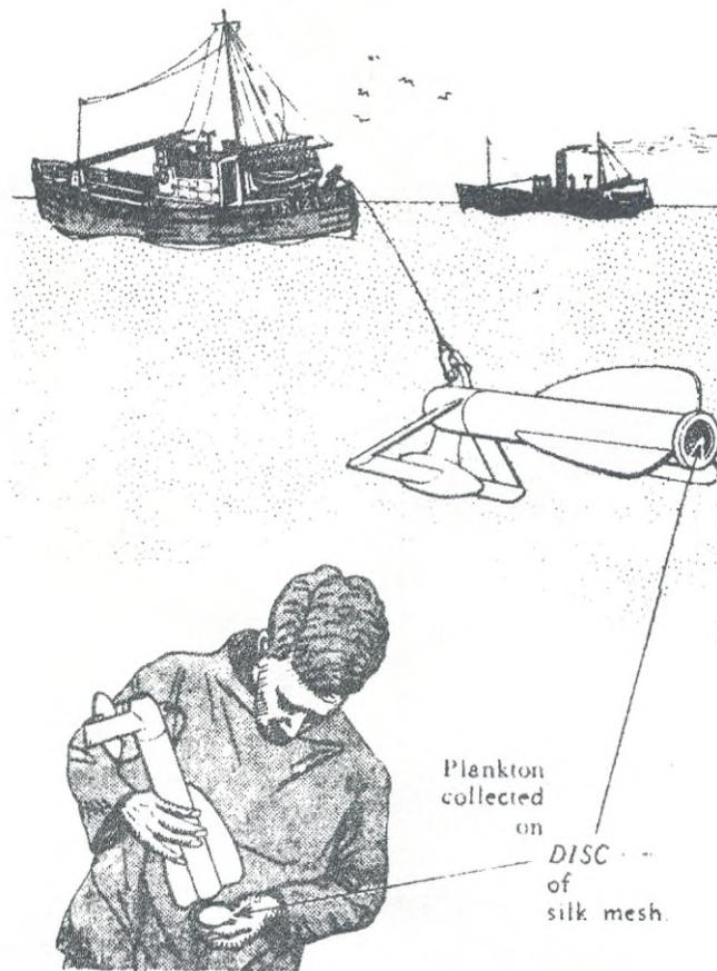
Fig.9. The Hardy Plankton Indicator, as used to sample plankton by fishing vessels working on the herring grounds (Fraser, 1962).
