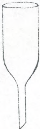
Fig. 1c. Adapter for Gooch Crucibles
