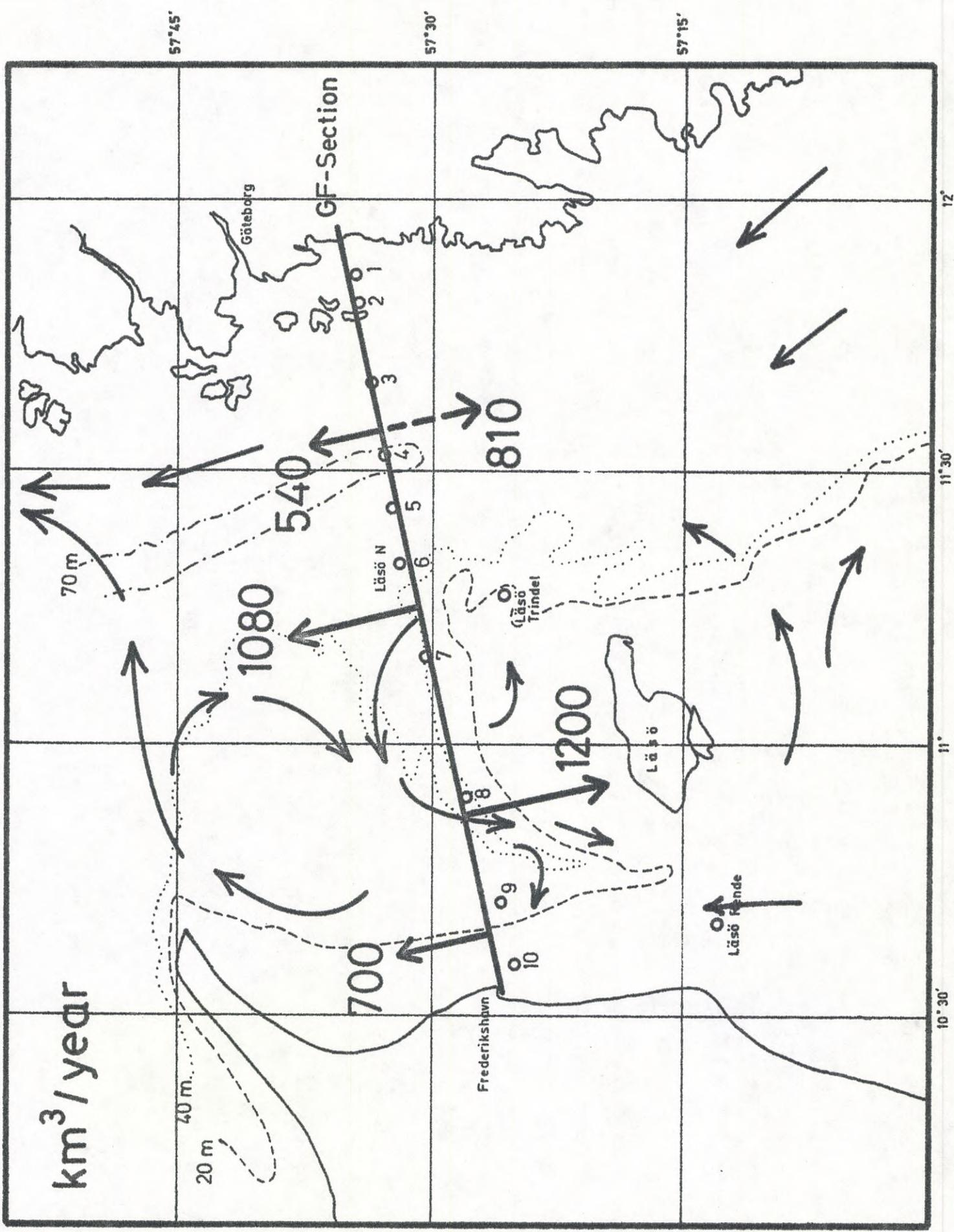
Water transports based on corrected current measurements to bring saltbalance
